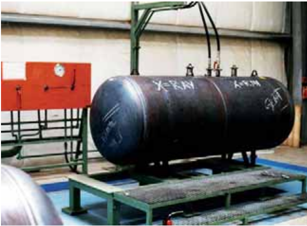
Hydrostatic Pressure Testing: on special, individual test benches
