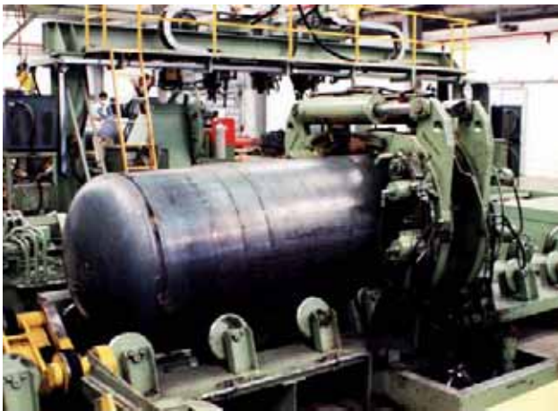
Assembly: domed ends and body are assembled on hydraulic devices.
